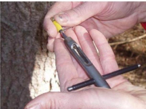
...and then the microcore goes in the slit of the tool
