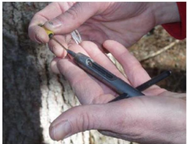
using the "extratcing needle" push lightly the microcore on the top ...
