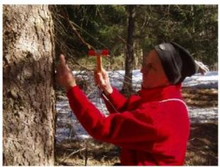
drive in the trunk the tool's blade using exclusively a **rubber** or **plastic** hammer.
